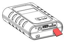
Install SIM card first (Chip facing down, Norch facing in) Power on the tracker.
